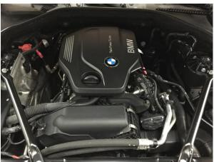
3. Find plug for rail pressure sensor. Disconnect it and connect box adapter between.
