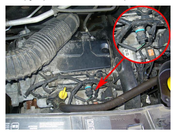
3. If box is equipped with yellow-red wire connect it to positive terminal in an engine compartment.
