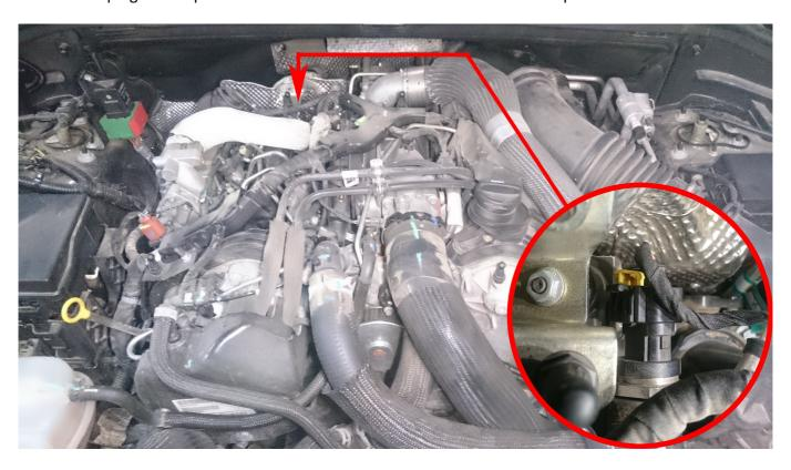
3. If box is equipped with yellow-red wire connect it to positive terminal in an engine compartment.
