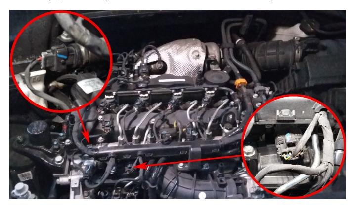
3. If box is equipped with yellow-red wire connect it to positive terminal in an engine compartment.
