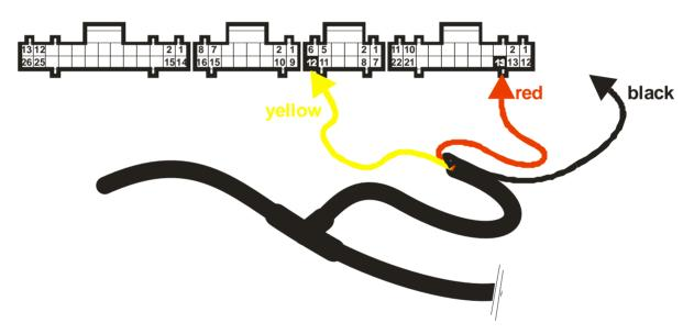
3. Connect black wire with fuse to fuel pump (typically red or gray wire).
